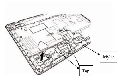
Figure 4-18 Removing Bluetooth
